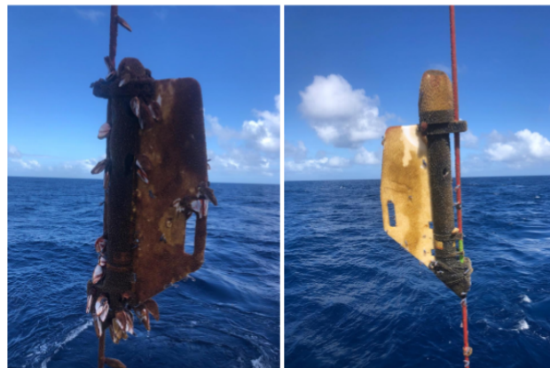
Recovered ADCP instruments at the end of a successful deployment at the 2°S, 140°W mooring at 23 m depth (left) and 68 m depth (right).
